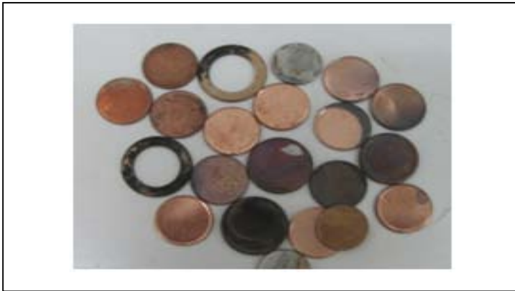
Figure 1. Samples of defective blanks and rings.
