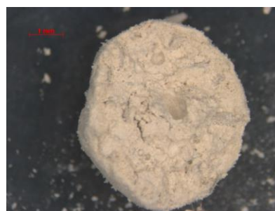
Figure 3: Pellet of palygorskite and transparent glue.
