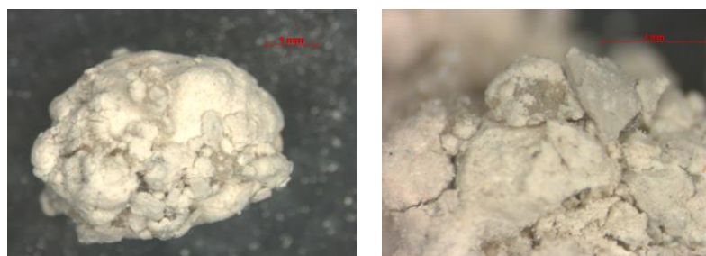
Figure 1: Pellets of palygorskite and granulated PVA.
