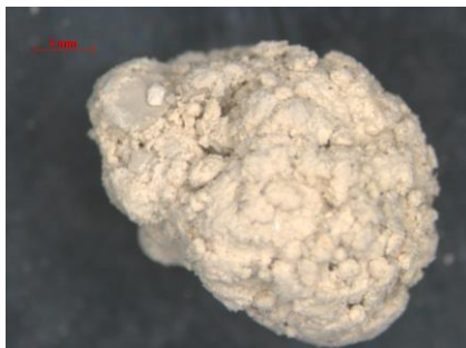
Figure 4: Pellet of palygorskite and glue mixtures.
