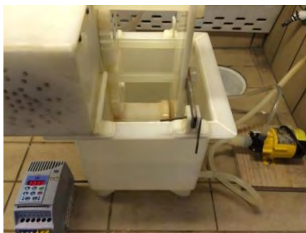
Figure 1: Reaction system for the leaching tests.
