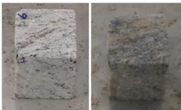
Figure 1: MSB 2 sample before and after 17 cycles of saline immersion and thermal shock.
