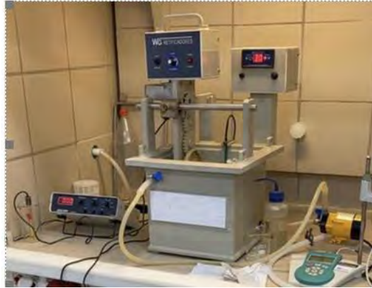
Figure 3: Reaction system used in the bio-extraction of base metals from electronic scraps.
